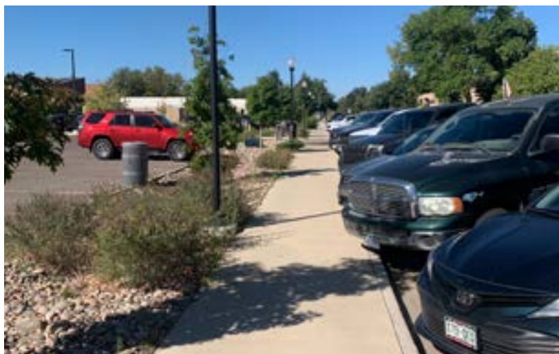
Image of an attached sidewalk without an amenity area
